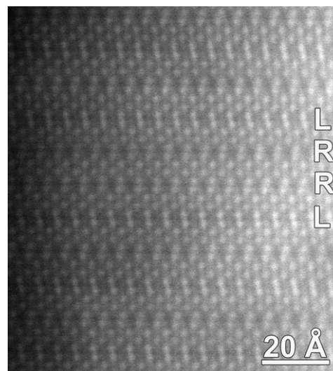
Fig. 6. HAADF-STEM image along [010] of an area showing defects in the L–R–L–R sequence of the layers.
